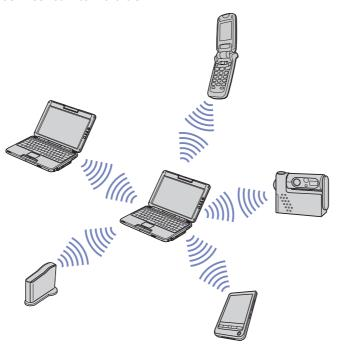
Do not simultaneously use the Bluetooth™ function and wireless communication devices which use the 2.4 GHz band such as a wireless LAN PC Card.
